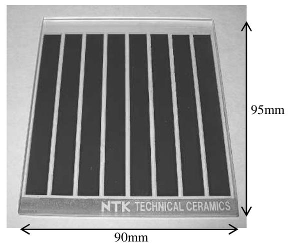
Fig. 2 Photograph of DSSC using ceramic substrate
