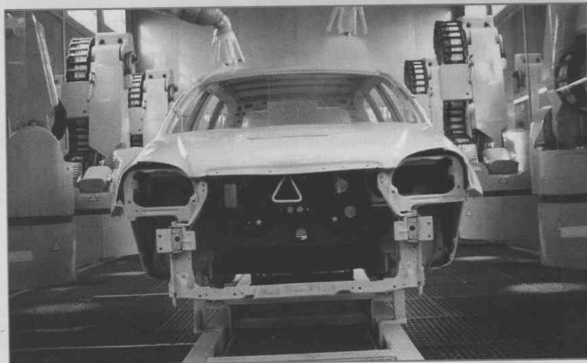
Figure 1. Shanghai General Motors' Excelle model - exclusive to the Chinese automotive market - finished using BASF waterborne basecoats (Image courtesy of BASF)
